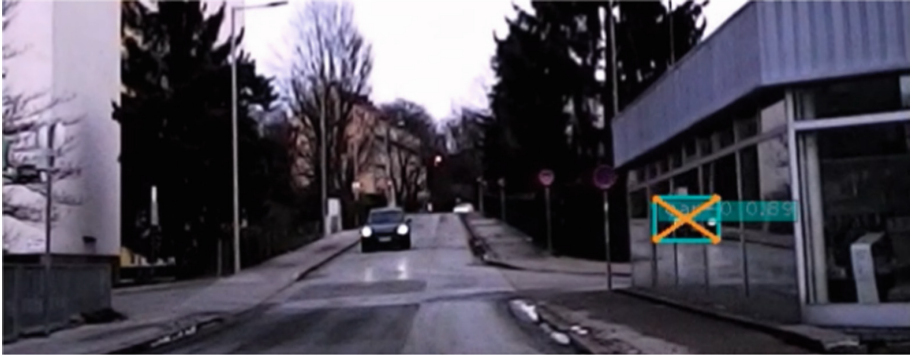
Fig. 1. Real-world example where the mirroring of an approaching object is detected instead of the actual object.
