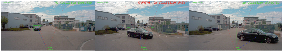
Fig. 5. Example result obtained from applying our ASP model on the A2D2 dataset. Left: no collision is expected with the detected object at time t_1 . Middle: on collision path at time t_2 . Right: critical situation resolved at t_3 .
