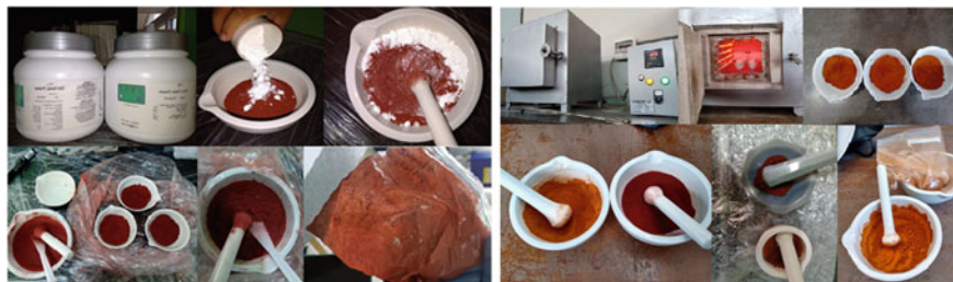
Fig. 1 Mechanical preparation and mortar grinding of raw materials and heat treatment or synthesis of zinc ferrites followed by their mechanical preparation for complete characterization
