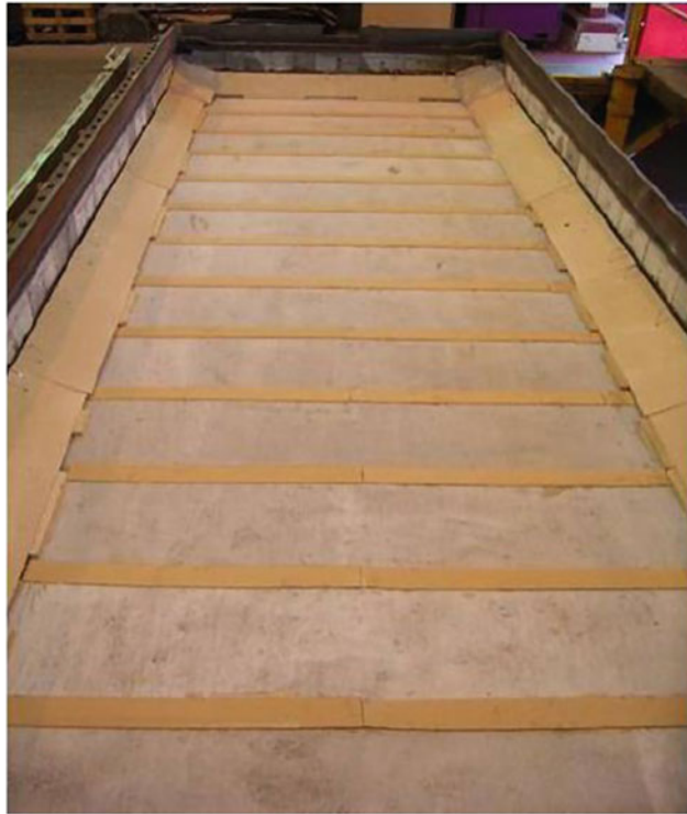
Fig. 13 Start-up protections of ECP2 cells showing insulation over the ram fillets and rammed slots
