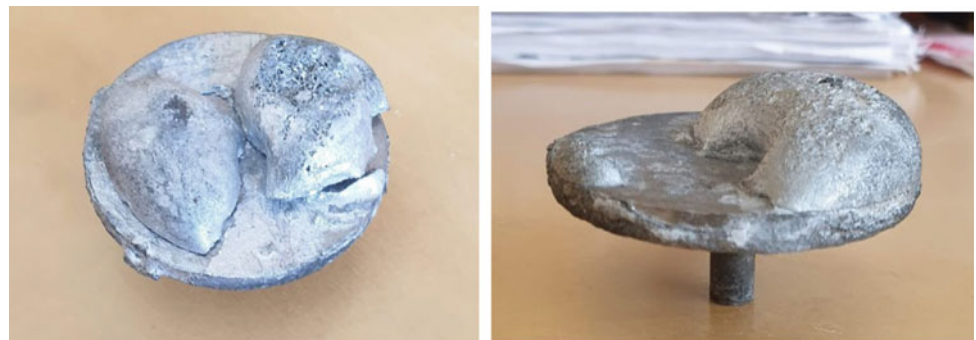
Fig. 6 Deposits using NaF-AlF 3 cryolite with no alumina feeding at 3 wt. % Mn, CR = 2.2, CCD = 0.9 A/cm 2 , t = 4 h, (left) T = 970 °C, (right), T = 980 °C
