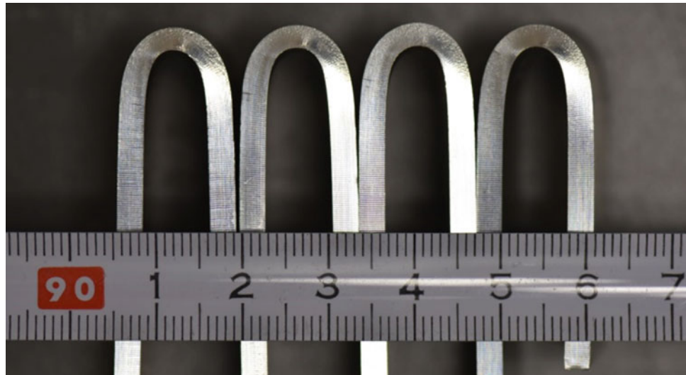
Fig. 5 Bending samples of 180° according to ASTM290 (radius N = 1 ) at different coil positions of alloy C transverse to the rolling direction
