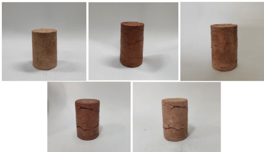
Fig. 7 Durability test on specimens
