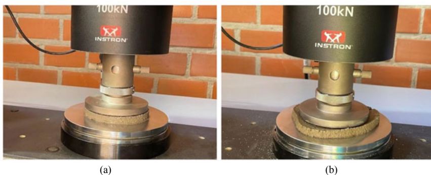
Fig. 4 Squeeze flow test apparatus: a before the test; b after the test
