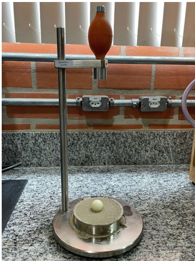
Fig. 3 Dropping ball test equipment
