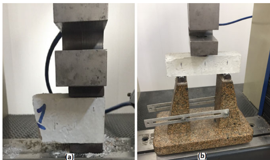
Fig. 2 Specimen: a compression; b flexural tests
