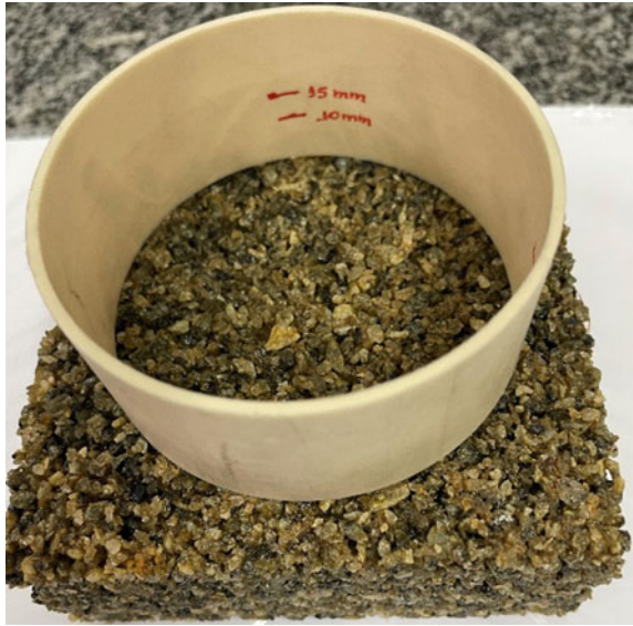
Fig. 2 Assembly of the test to determine the permeability coefficient (a)
