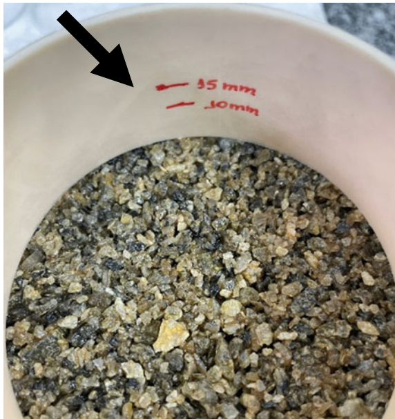
Fig. 3 Assembly of the test to determine the permeability coefficient (b)
