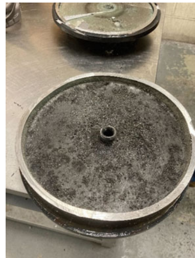
Fig. 8 Cut open condenser of the one-effect distiller
