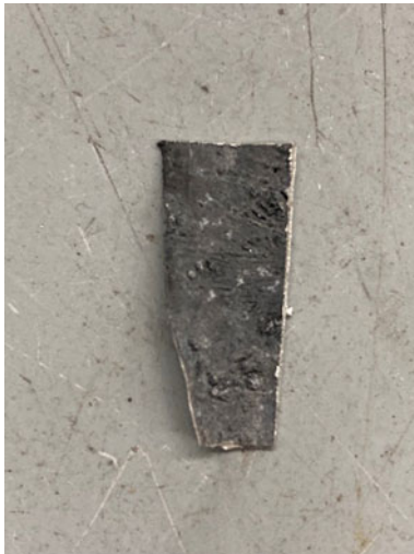
Fig. 9 Black oxidation coating on top surface
