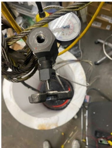
Fig. 2 Vacuum gauge and valve setup
