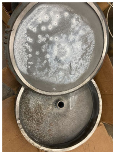
Fig. 4 Mg nucleation at the condenser (top plate)—unsuccessful distillation
