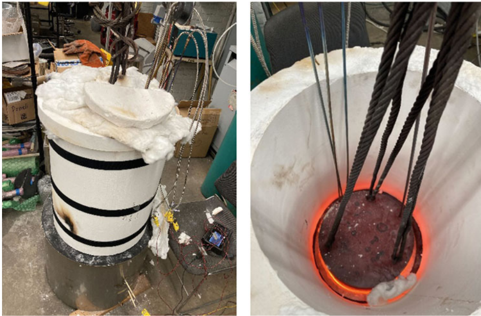
Fig. 5 10" AZ91 distiller setup before (left) and during (right) the final successful experiment
