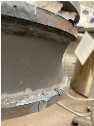
Fig. 7 Shrinkage deformation of the evaporator in the final experiment
