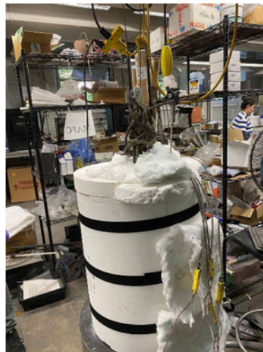
Fig. 3 10" distiller setup inside the insulation fiber
