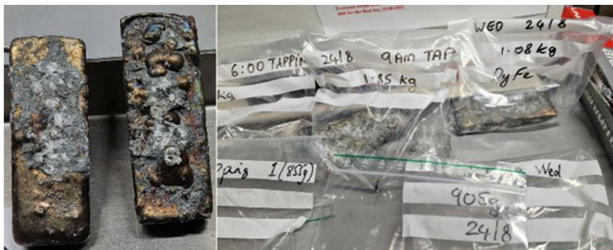
**Fig. 4** DyFe metal alloy ingots from the trials showing some frozen electrolytes on them
