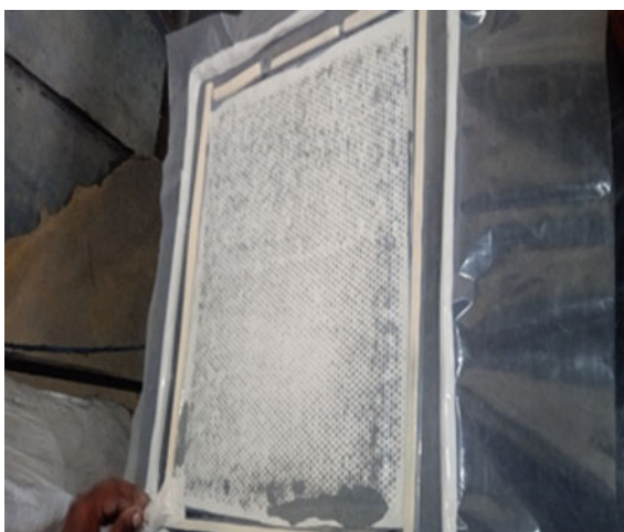
Fig. 1 Vacuum bag molding process
