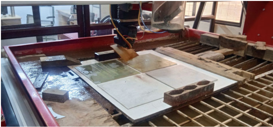
Fig. 3 Abrasive waterjet cutting of fabricated specimens
