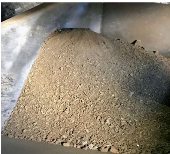
Fig. 10 Sulfated dust reclaimed in convection section
