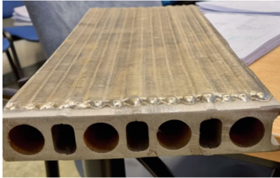
Fig. 16 Double omega panel with overlay cladding
