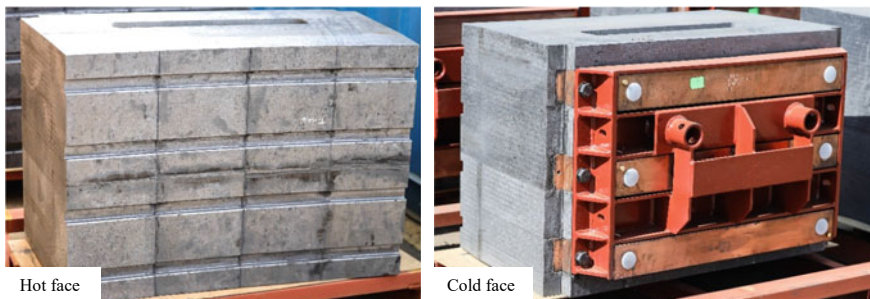
Fig. 5 Furnace 1 composite copper-graphite cooler design
