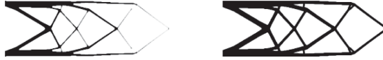
(a) Increased \eta \rightarrow eroded design (b) Decreased \eta \rightarrow dilated design
