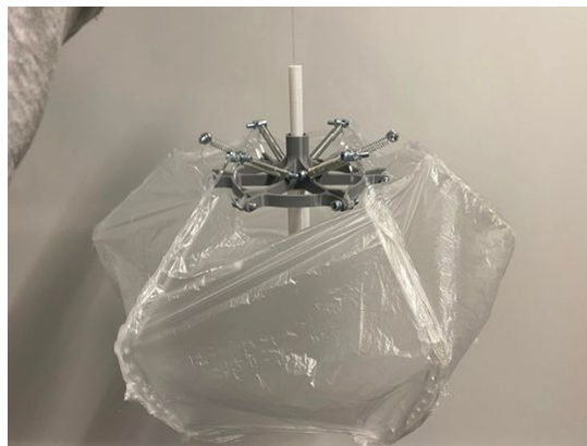
Fig. 6. The final state of the prototype with the plastic bag simulated the net functionality.
