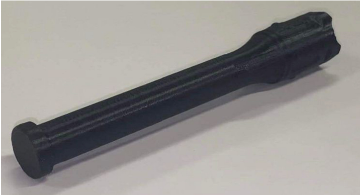
Fig. 1. FDM printed model of NASA's sample tube to test gripper compatibility
