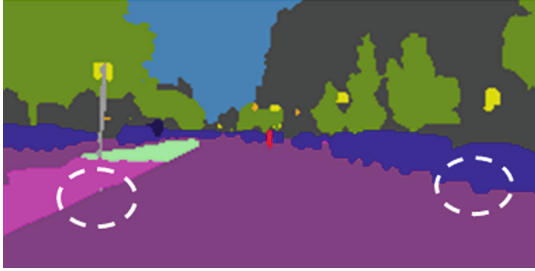
Fig. 7. A semantic segmentation input mask \bar{\mathbf{m}}_t from \mathcal{D}_{\text{val}}^{\text{BDD-MOTS}} showing different semantic classes. The left white encircled region portrays the proximal occurrence of class sidewalk ( s = 2 ) near to class road ( s = 1 ). Similarly, the right white encircled region portrays the proximal occurrence of class road ( s = 1 ) near to class car ( s = 14 ).
