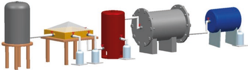
Fig. 6 Alternative C: pyramid solar still coupled with a cylindrical absorbent bed with a fin tube heat exchanger
