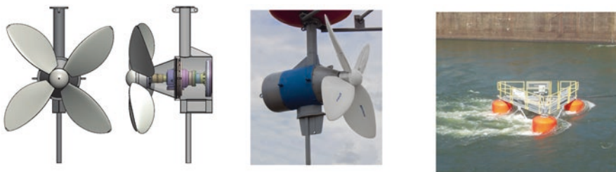
Fig. 1 HK-10 turbine: front and lateral views of the conception model, photo and field assembly
