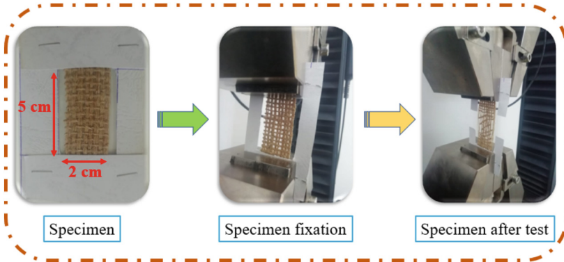
Fig. 2. Fixation system of Jute fabric specimen.
