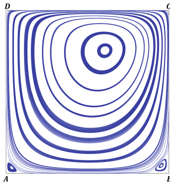
Fig. 3. Streamlines of subsonic flow in a square cavity for Re = 100 and for Ma = 0.1
