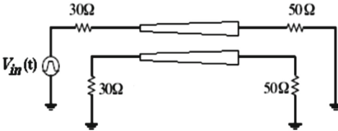
Fig. 4. Two interconnects test circuit with linear loads.
