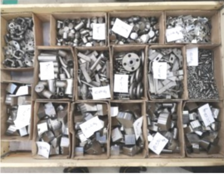
Fig. 1. Scraps of green 316L stainless steel.
