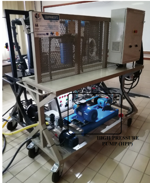
Fig. 1. Pilot RO desalination plant. E5DES (MAC2/1.1a/309) Project
