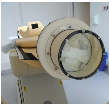
Fig. 2. Head-16 Simulator used in daily MX 16 scanner's quality tests at the CHC-UFPR.
