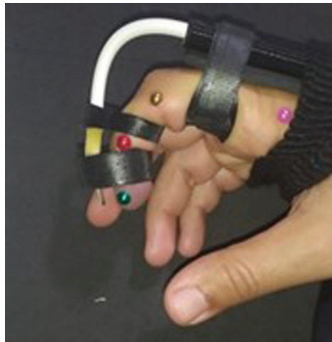
Fig. 2. Fixed PP assembly - the cable guide (black) is fixed on the proximal phalanx (PP) in order to constrain MCP joint rotation
