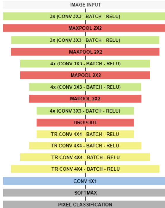
Fig. 2. CNN architecture used for semantic segmentation of TB bacilli.
