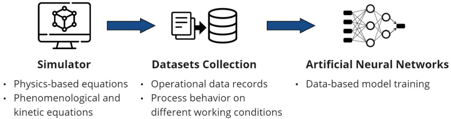
Fig. 3. Froth flotation virtual model development: Hybrid approach methodology.
