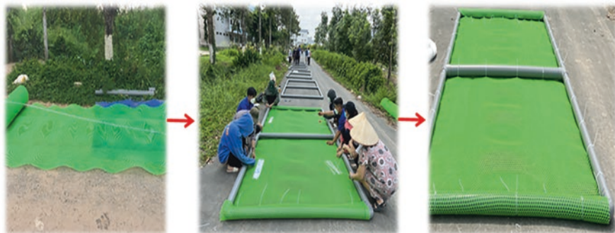
Fig. 10.10 The process of fixing the net to the raft frame
