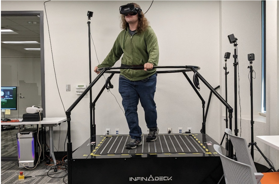
Fig. 1. Infinadeck omnidirectional treadmill
