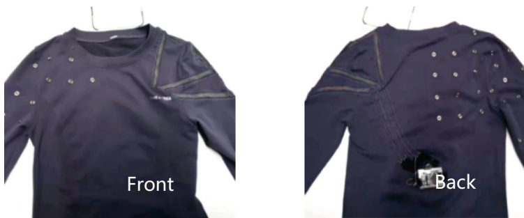
Fig. 2. Smart garment prototype with fabric strain sensors
