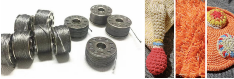
Fig. 2. Silver-plated yarn and fabric pieces woven with both conductive yarn and baby yarn.
