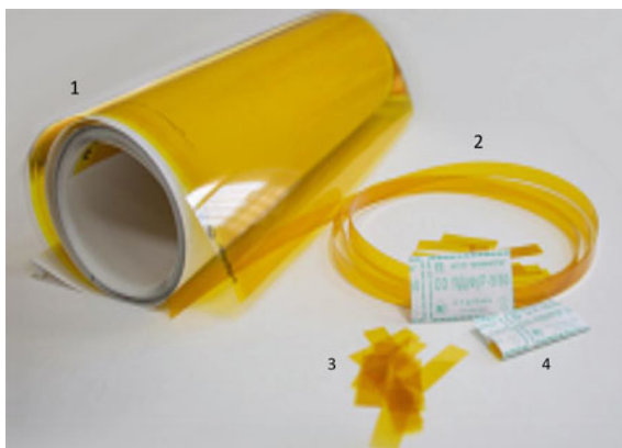
Fig. 1 The design of films-blanks of reference materials of absorbed dose
