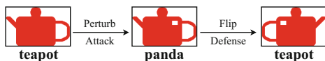
Fig. 1. The flip symmetry defense against zero-knowledge adversaries reverts adversarial images to their correct classification by horizontally flipping the images before classification. The defense classifies non-adversarial images in the same way.
