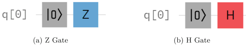
Fig. 1. Z Gate applied to a |0\rangle state and H Gate applied to a |0\rangle state
