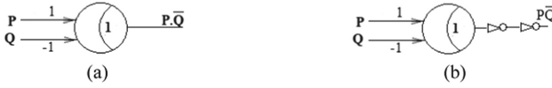
Fig. 8. (a) Threshold gate of P = P\bar{Q} . (b) Threshold gate of A\bar{B} using 2-buffers
