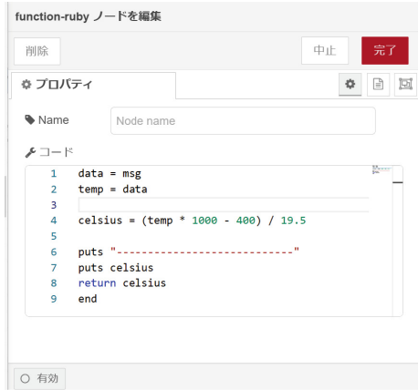
Fig. 5. Ruby function node, contains ruby code for converting from voltage to temperature
