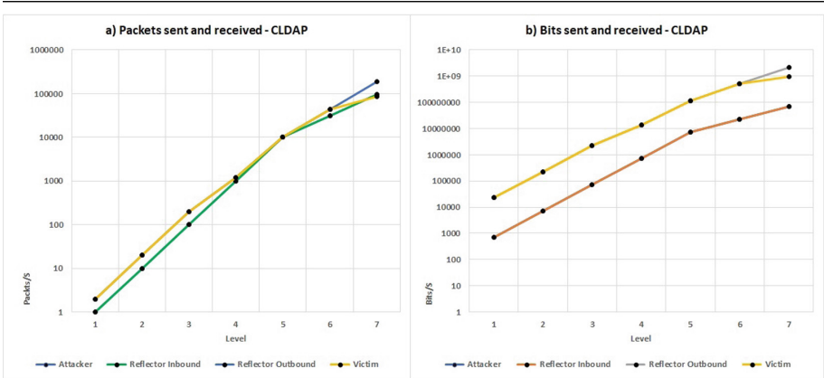
Fig. 1. Packets and Bits sent and received per second - CLDAP
