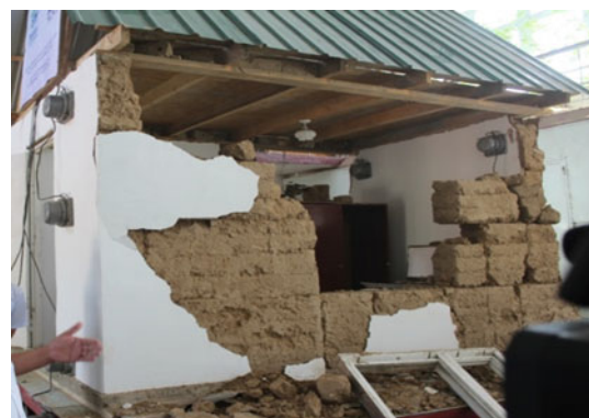
Fig. 1 General view of the model of the house «sockmo» after the experiment
