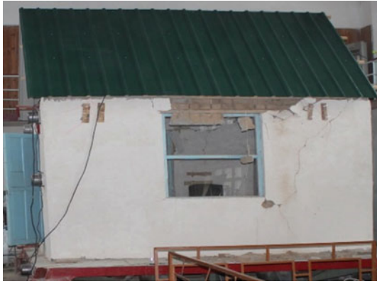
Fig. 2 General view of the model of the house, made of brick raw, after the experiment
