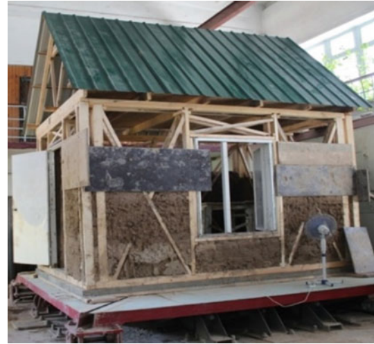
Fig. 3 The process of construction of a model house of wooden frame «synch»
