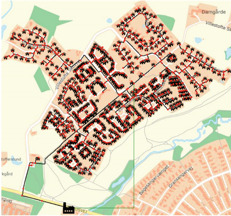
Fig. 4. Visualisation of DHS implemented in the LHN model. The substation located at the bottom supplies the 648 consumers through the pipe network, which represents the real configuration of the DHS. Red dots represent the nodes connecting the pipes and black houses represent the individual consumers. (Color figure online)
