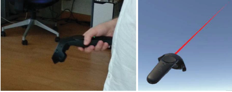
Fig. 5. Pointing and steering with Vive controller.
