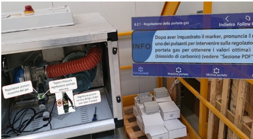
Fig. 3. Example of an “AR scene” of the developed MRTD about gas flow adjustment.
