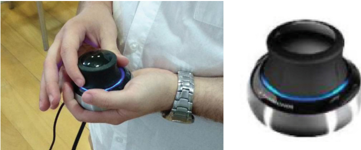
Fig. 3. Our GDS-3DMouse technique is based on a compact 3Dconnexion device.
