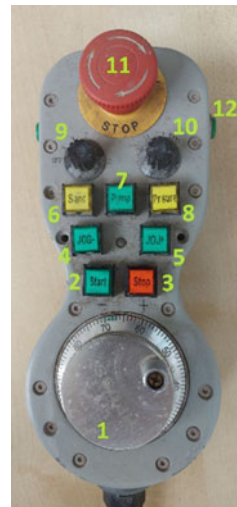
Fig. 11 Machine hand panel: Emergency button (1), NC stop (2), NC start (3), Reset (4), Feed rate override (5), Pressure override (6), High pressure display (7)
