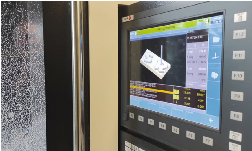
Fig. 44 Simulating the program in the milling machine
