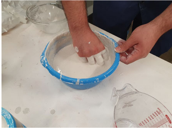
Fig. 8 Preparation process of the gypsum plaster
