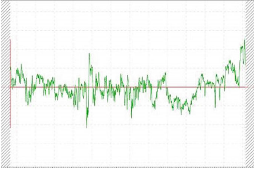
Fig. 14 Example of a roughness profile measured on the internal surface of an investment cast and subsequently polished ring
