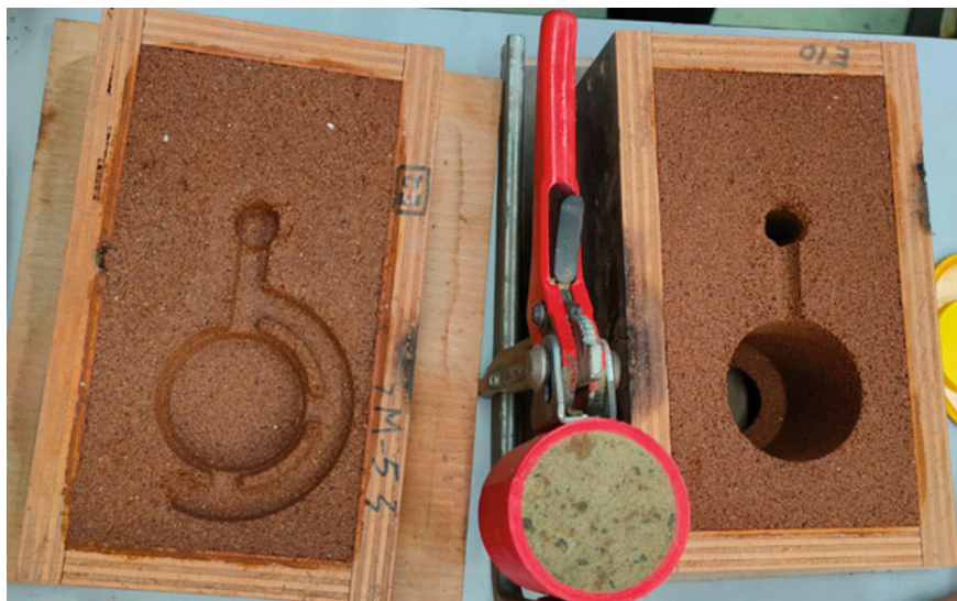
Fig. 22 Drag, core box, and inferior cope
