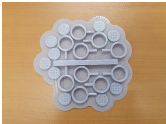
Fig. 3 Group of 3D printed wax patterns of the rings, of decorative motifs and of the central pillar of the wax tree
