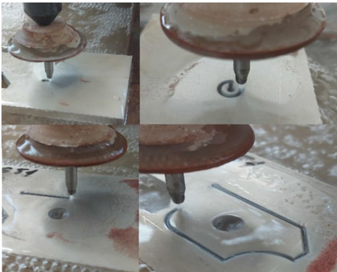
Fig. 30 AWJ cutting progress
