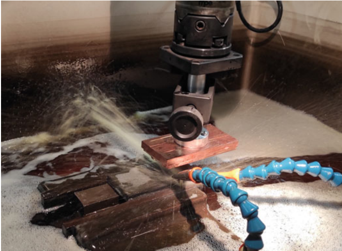
Fig. 52 Starting the EDM process: verifying the cleaning method
