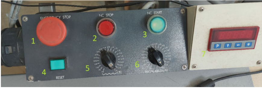
Fig. 11 Machine hand panel: Emergency button (1), NC stop (2), NC start (3), Reset (4), Feed rate override (5), Pressure override (6), High pressure display (7)
