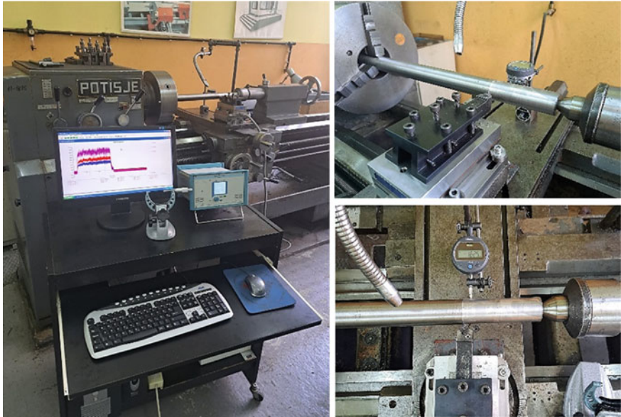
Fig. 7 Measuring setup on the universal lathe
