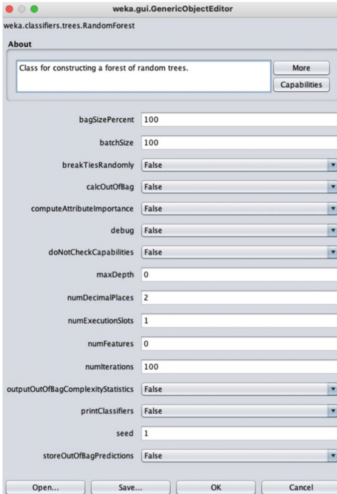
Fig. 5 Weka interface to modify the hyperparameters of the RF model
