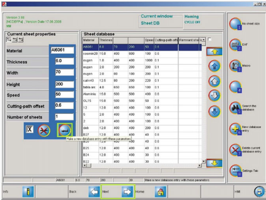
Fig. 21 Adding the material in the database
