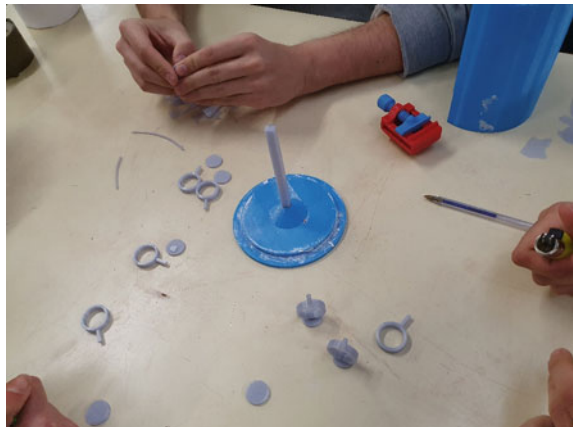
Fig. 5 Building process of a wax tree
