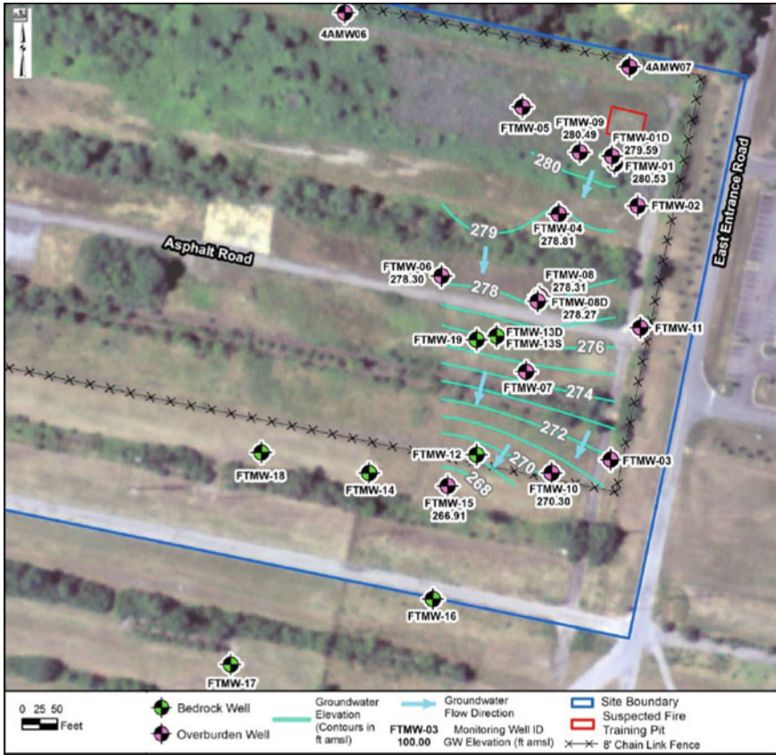
Fig. 7.7 Monitoring well layout and groundwater flow in overburden aquifer
