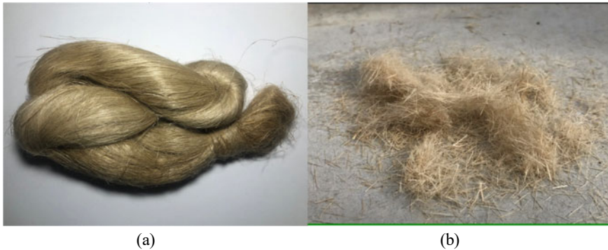
Fig. 4 Test fibers: a tow linen, b prepared, chopped test fibers
