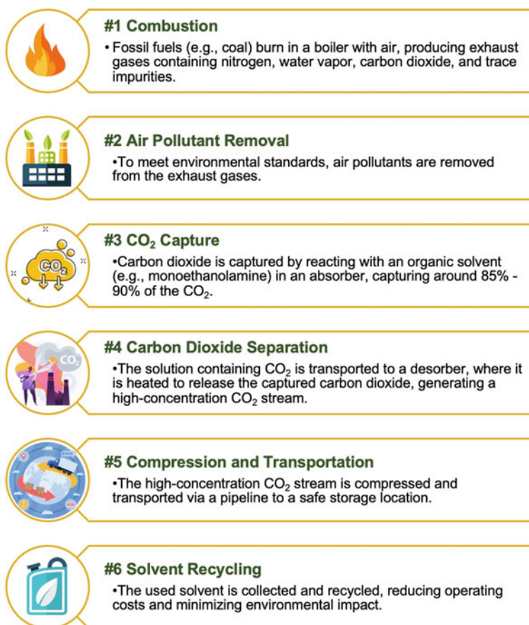
Fig. 17.4 Post-combustion process for CO 2 capture process
