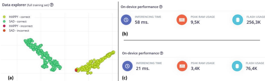
Fig. 3. a Classified training data mapped on a reduced order 2-D space. Summary of the estimated on-device performance of the network on the target MCU for b 32-bit and c 8-bit quantized data.
