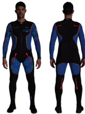
Fig. 1. The suit with detailed flexometers (in red) and electrodes (in blue), for a limited number of sensing and stimulation points.
