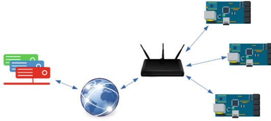
Fig. 1. Typical structure of an IoT system: Servers, on the left, are connected through internet to a gateway (black box) which in turn communicates with end-nodes
