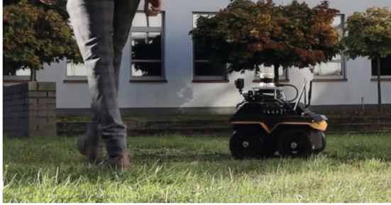
Fig. 3. Jackal stops after obstacle is too close, as identified in TeSSLa. Full video at https://www.tessla.io/blog/rosBridge/
