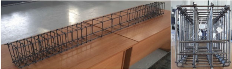
Fig. 1 Scheme of reinforcement of reinforced concrete structures: reinforcement \text{\O}6 mm class A240 (1); reinforcement \text{\O}10 mm class A500s (2); reinforcement \text{\O}5 mm class Vr500 (3); equal-shelf corner 100 \times 10 mm (4)
