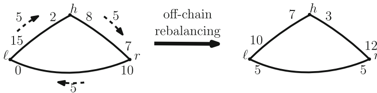
Fig. 1. Example of off-chain rebalancing with users \ell , h , and r . The graph on the right depicts the channel balances after off-chain rebalancing.
