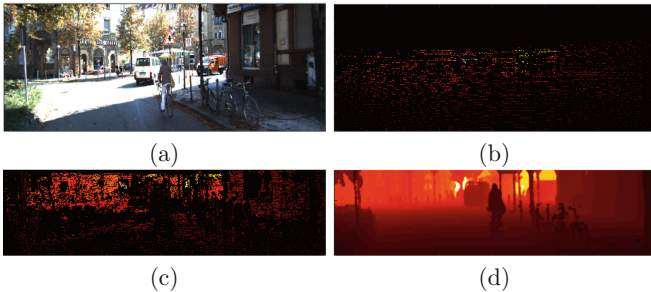
Fig. 7. Examples of completed depth maps. (a) reference color image. (b) Available sparse depth map. (c) ground truth. (d) Completed depth map.
