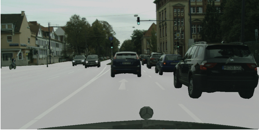
Fig. 1. Drivable area. The region-of-interest are roads and sidewalks, which are highlighted in white in this image. We employed semantic segmentation inference to identify the contours of this area. Any anomaly completely enclosure within the drivable area is a road obstacle for this research.
