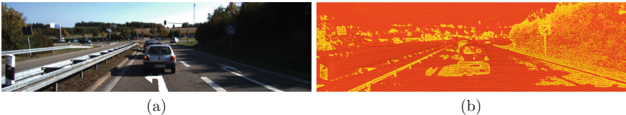
Fig. 4. Example of balance term \gamma(\mathbf{x}) computer for an urban color reference image. (a) color reference image. (b) color-coded balance map \gamma(\mathbf{x}) larger gamma values are color-coded with yellow and orange representing \gamma = 0.46 .
