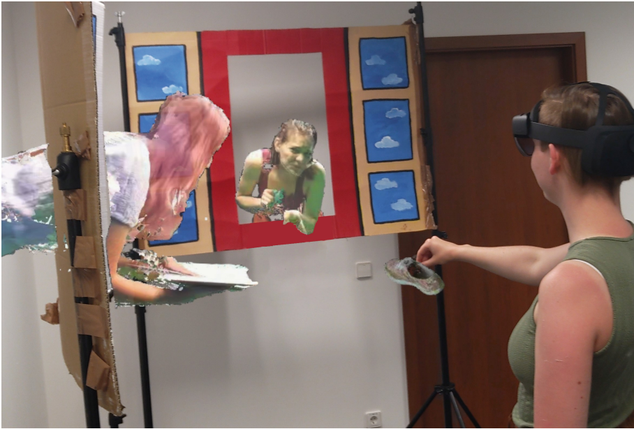
Fig. 1. Handing back the virtual shoe: interaction with volumetrically filmed virtual figures appearing in a physical cardboard window frame, captured by a second HMD.
