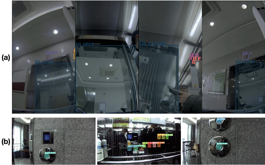
Fig. 5. Dataset overview. (a) Indicator dataset: object detection dataset is tailored to capture the basic status of an elevator. (b) Button dataset: instance segmentation dataset designed to identify points of interaction between the robot and the elevator, facilitating precise and successful task execution.
