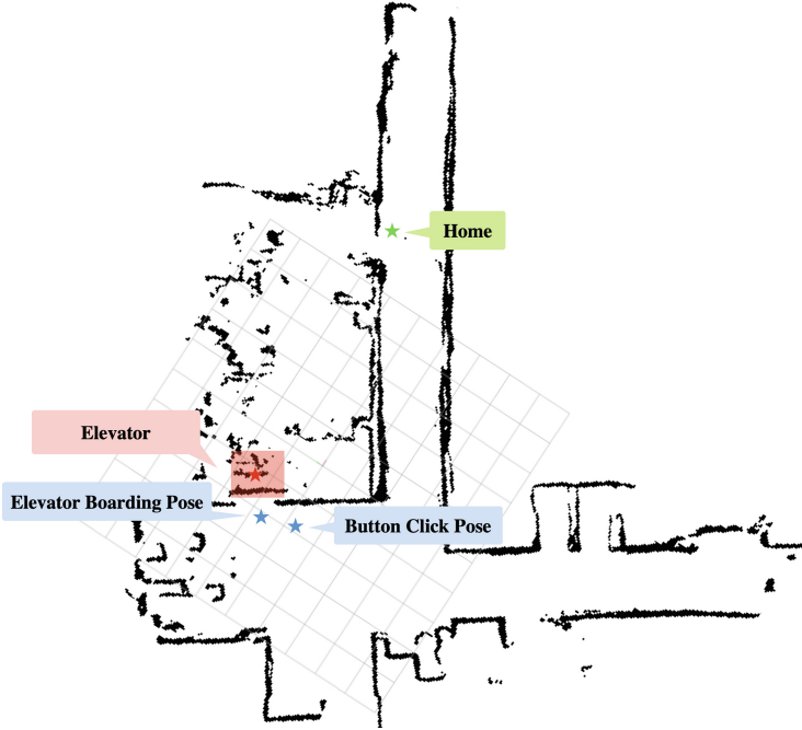
Fig. 6. Occupancy map of Woojung Hall of Informatics. This figure illustrates the constructed occupancy map of the 6th floor of Woojung Hall of Informatics at Korea University, which serves as the operational landscape for all our real-world robot experiments.
