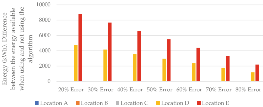
Fig. 3.18 Energy available depending on the error in energy consumption estimate when using 44 engineers only for destinations D and E
