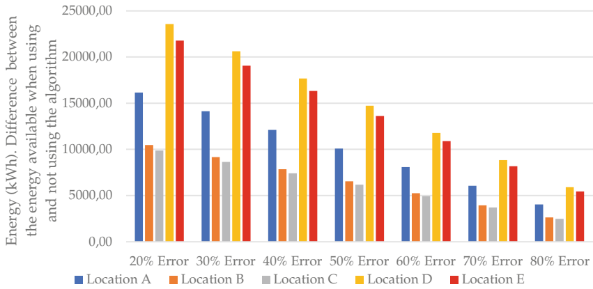
Fig. 3.16 Energy available depending on the error in energy consumption estimate when using 400 engineers
