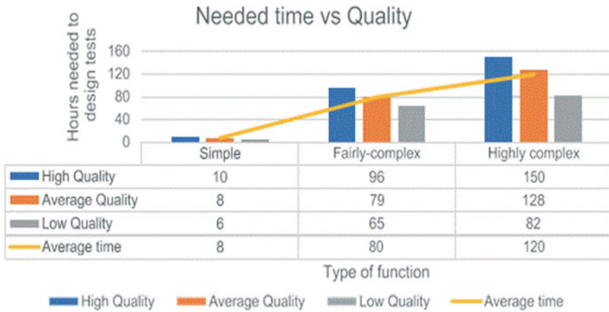
Fig. 2.41 Engineering hours spent for test design depending on the type of SM to be validated in black-method
