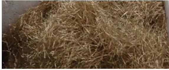
Fig. 7.1 Representative sample of the employed steel fibers ( Dramix ® OL 13/0.20 ). Adapted from Feo et al. (2020)
