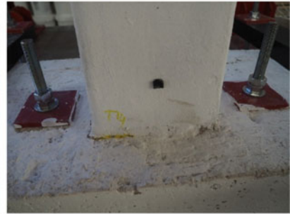
b. High-strength steel rods and profiles for connection between foundation and shake table
