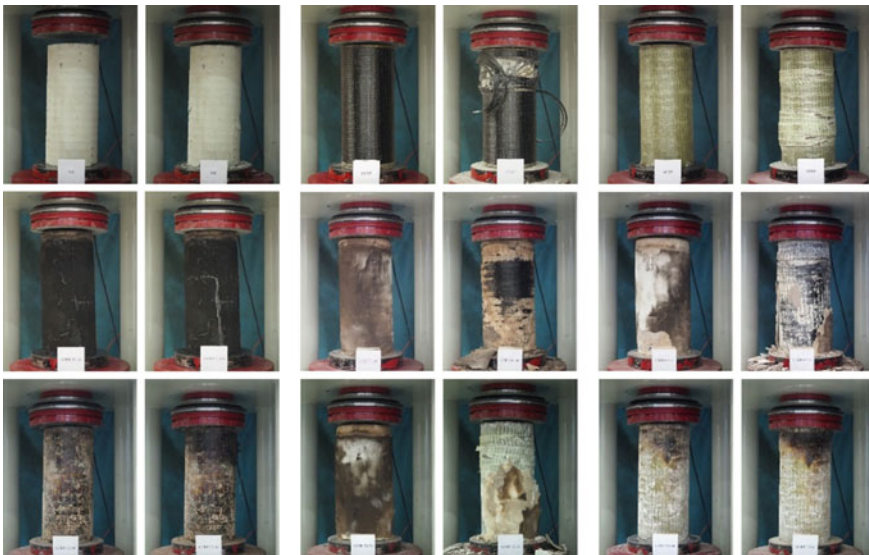
Fig. 9.5 The overview of the compressive strength of some specimens before and after fire tests
