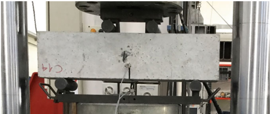
Fig. 7.4 Experimental set-up for 4-point bending test. Adapted from Ismail and Ohtsu (2006).
