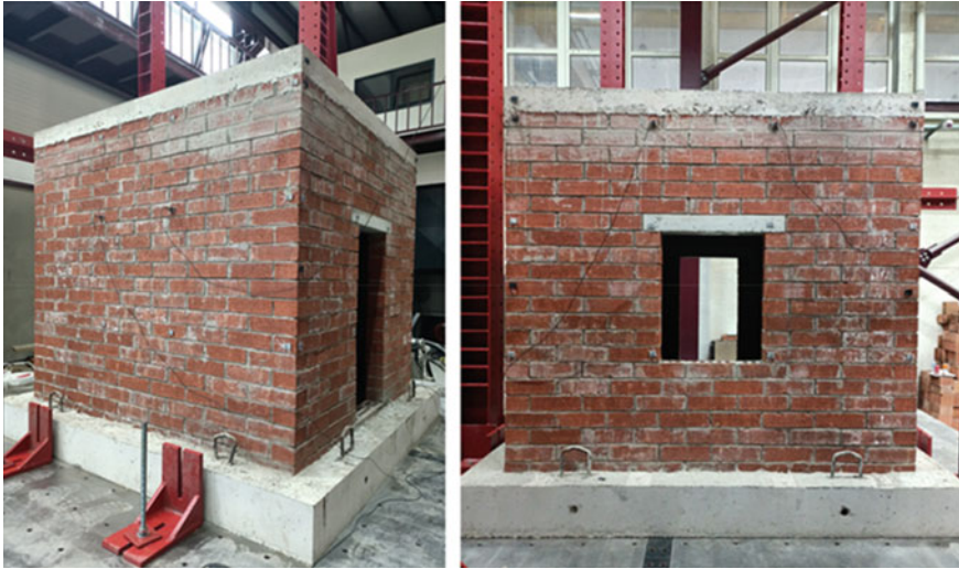
Fig. 13.1 The masonry model utilized as a case study
