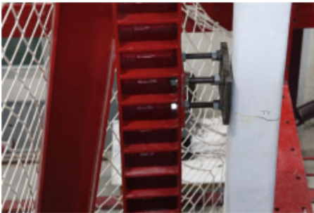
c. Adjustable collision element and collision wall
