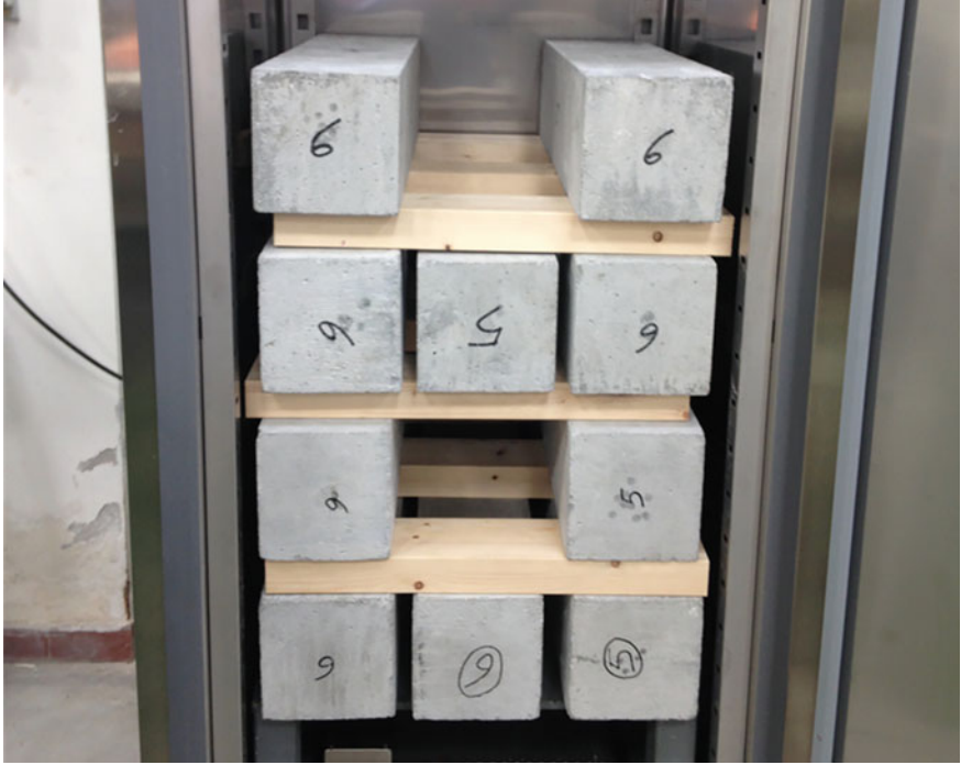
Fig. 7.3 Freeze-thaw cycling apparatus. Adapted from Ismail and Ohtsu (2006)
