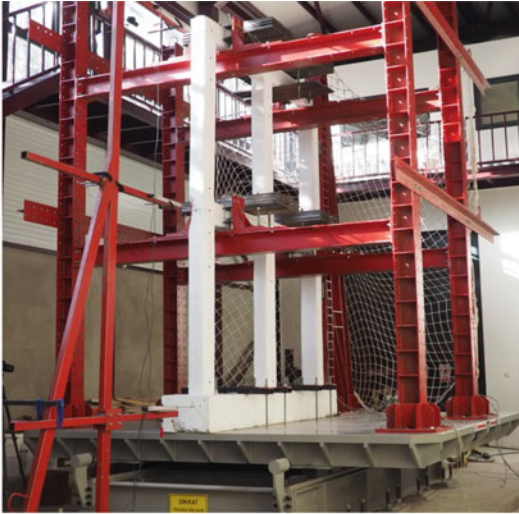
a. General view of the experimental setup for shake table tests
