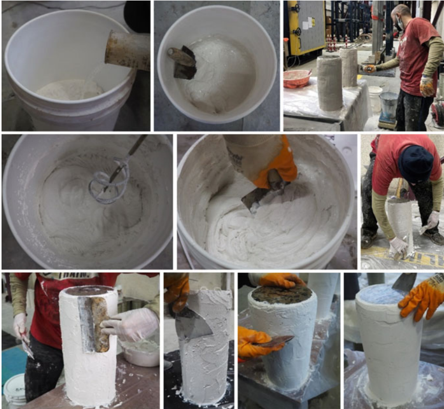
Fig. 9.3 Preparation and application of the System C components
