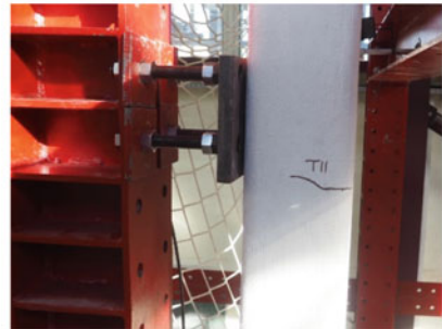
c. Adjustable collision element and collision wall
