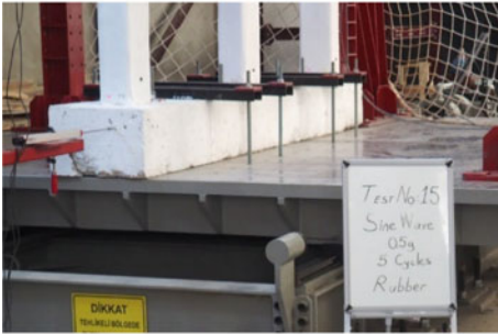
b. High-strength steel rods and profiles for connection between foundation and shake table
