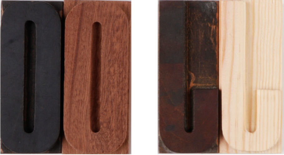
Fig. 7. Detail magnification - On the left, are the reference types, and on the right, are the types reproduced in the pantograph.
