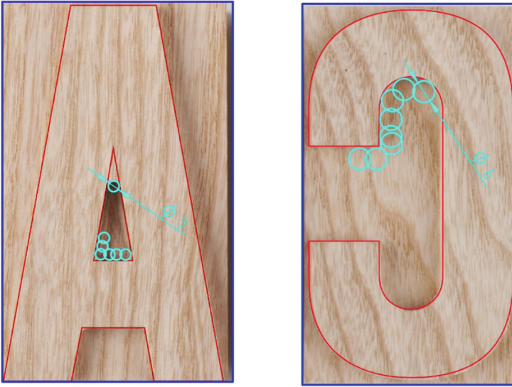
Fig. 8. Detail magnification – The figures show an image of the ash types made on the CNC machine, digitally outlined with the original shape (red), and marked with the diameter of the shape of the cutter used (cyan blue). In the A type, the inner vertices in the letter anatomy are slightly rounded, compared to the C type on the right, where the typeface design is unchanged due to the letter’s concave angles.
