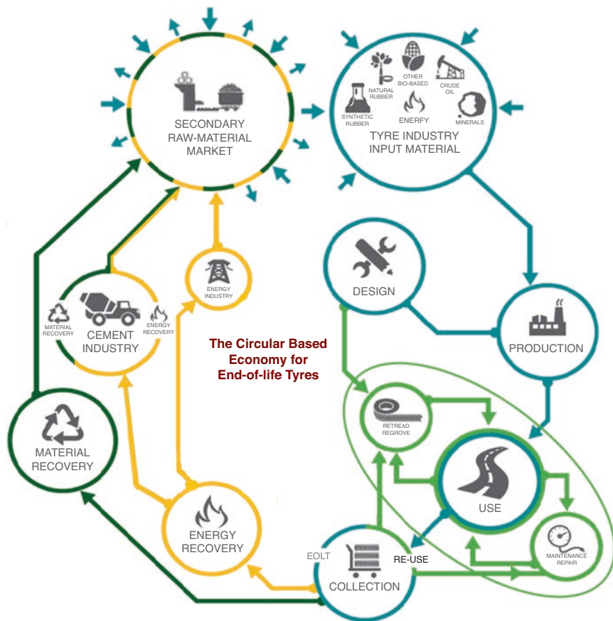
Fig. 3 A typical circular-based economy cycle for end-of -life tires (EOLT) (ERJ 2020), (Dobrot et al. 2019), (ETRMA 2017, 2019b)
