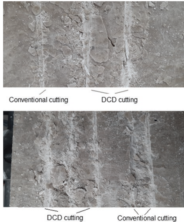
Fig. 6 Comparison of the rock chips and fragments between the DCD and conventional disc cuttings
