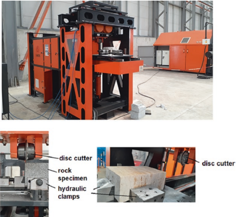
Fig. 3 General view of the DCD technology prototype and an oscillating single disc cutter
