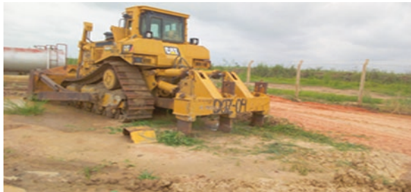
Fig. 2 A crawler equipment with three tine rippers at field site workshop
