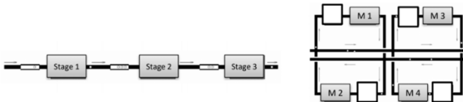
Fig. 6 Comparison of Flow and Job Shop. Source: Own representation according to Zimmermann and Stache (2001) [11].
