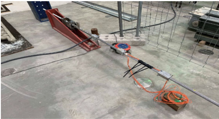
Fig. 6 Fiber optical sensors installed on the conductor
