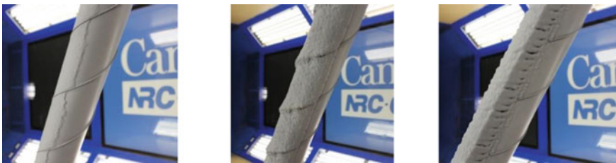
Fig. 2 Views of the cables with simulated ice in the NRC 2 × 3 m Wind Tunnel: cable 1 (left), cable 2 (center) and cable 3 (right)
