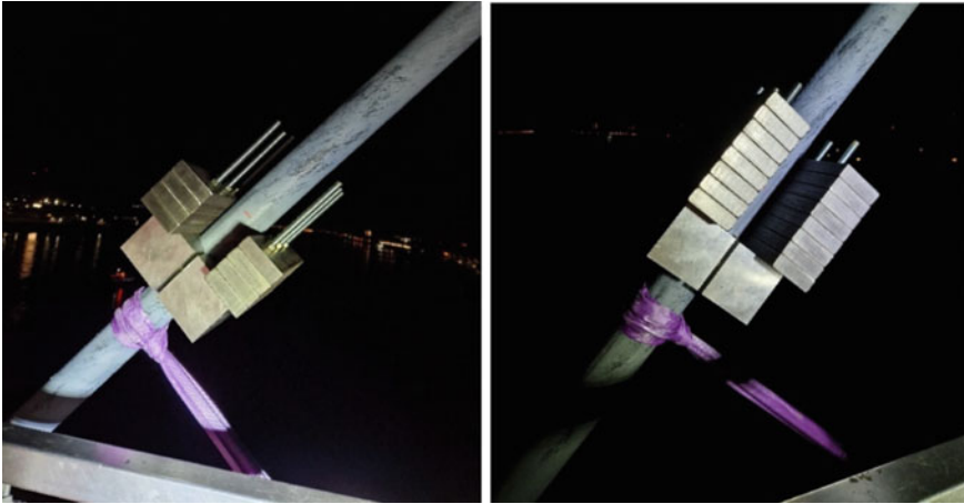
Fig. 3 Additional point mass attached to the cable. The left figure indicates the light weight (46.56 kg) and the right picture the heavy weight (82.28 kg)
